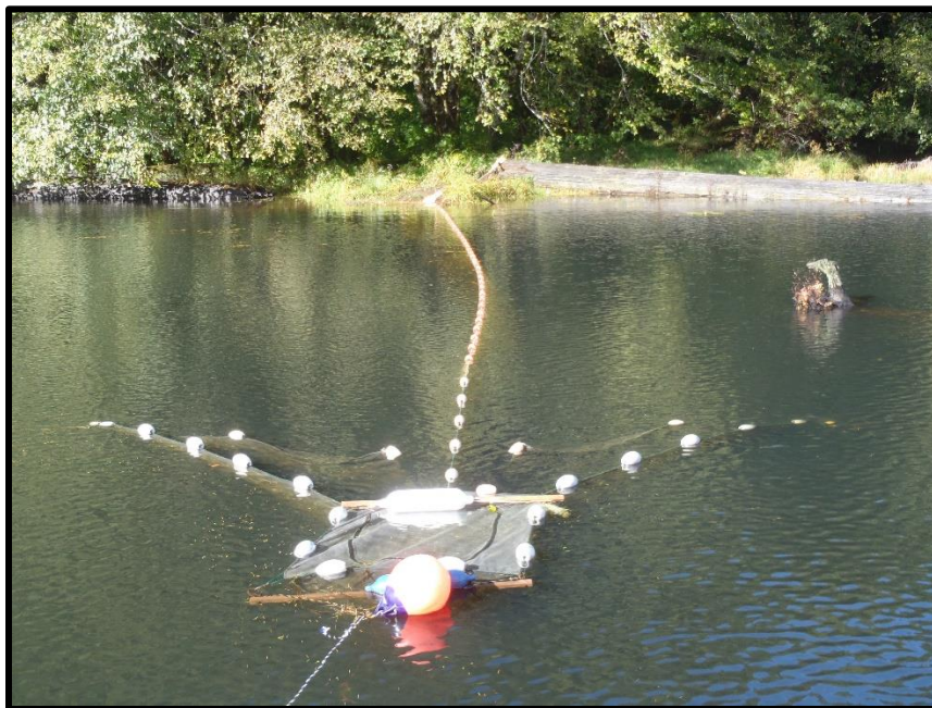
Figure 3. Miniature floating Oneida Lake Trap deployed in Hult Reservoir, October 2017.
