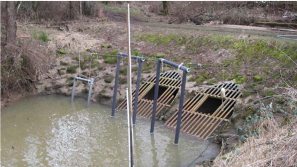
Figure 8. Antenna configuration at the upstream (A) and downstream (B) sides of the SWCS array.
